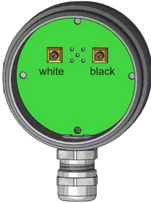
Probes with process connection have sockets (Y70) in the head. To connect, loosen the lid, insert the plug connection via the cable gland and connect it to the appropriate sockets. Here the sockets are marked with the colour coding corresponding to the evaluation unit. You will find suitable plug connections in our accessories programme.
