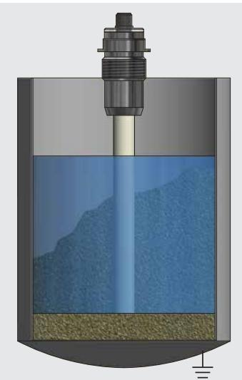
The patented 3-electrode measuring principle includes the container in the measurement. The container must therefore be made of metal or an additional electrode, e.g. metal foil or metal rod, which at least covers the measuring range, must be attached to the container. (Length of foil  $\geq$  probe length). The resulting large measuring volume is the reason why deposits on the probe surface are practically irrelevant for the measurement.
