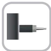
**For flush mounting in metal or other materials.** These sensors can be mounted close together and are specially designed for contact-less detection of solids or liquids through non-metal containers (max. wall-thickness 2 mm)
