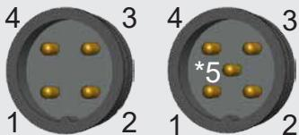
The protective earth connection (pin 5) is only present on sensors with metal housings and EST protected devices.
